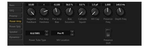
NEGATIVE FEEDBACK – Controls the amount of negative feedback in the power amp. The feedback decreases output impedance, causing the amp to react less to the speakers ("damping"). Higher values give a brighter, tighter, punchier sound but can be harsh at very high MASTER levels. Lower values give a smoother, loose and gritty sound and feel.
