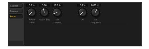
ROOM LEVEL/SIZE – Determines the level and size of room reverb that is built into the cab block. Increase to add room ambience to the sound.
