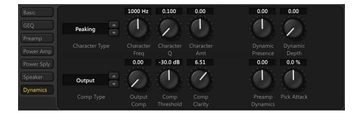
CHARACTER TYPE – Selects between a shelving behavior, peaking behavior, and Dynamic behavior. (With Dynamic, the character settings are engaged by playing harder. It can be used to fatten or scoop the tone as a function of picking strength.)
