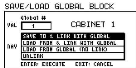
*Make a mental note of the name (and if there is one, the number) of the block type you are saving, shown in the upper right of the SAVE/LOAD screen (“CABINET 1” in the example above).*
