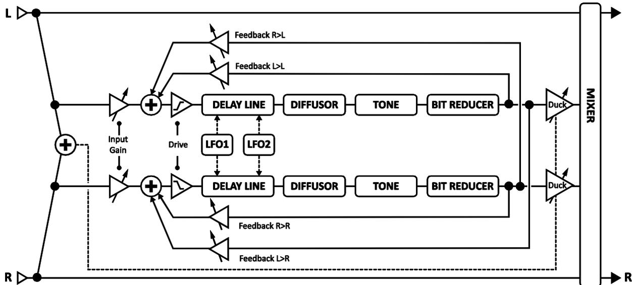
**TIME L, TIME R** – Dual parameters to set the time of the left and right delay lines. When **TIME** is shown in parenthesis, it is being set automatically by the **TEMPO** parameters (see below). Set **TEMPO** to “NONE” to regain manual control.
