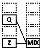
In the second example, the level of Effect **Q** would be controlled by the mixer’s CHANNEL 2 **LEVEL/GAIN** control, because **Q** is on row 2. Effect **Z** would be controlled by Channel 4, because Z is on row 4. The location of the mixer never matters, only the location of blocks connected to its inputs!
