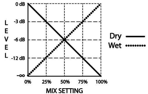
**LEVEL** – As you would expect, the **LEVEL** controls set the output level of a block. Almost all **LEVEL** controls have a range from -80.00 to +20.00 dB. Exceptions include the Compressor and Filter (+/-20.00 dB) and the Drive, which ranges from 0-10 dB.
