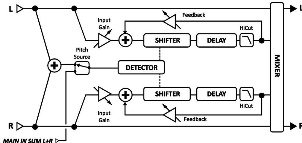
**INPUT MODE** – Specifies whether the incoming signal should be processed in stereo (as shown in the block diagram above) or summed to mono and then sent to both voices.
