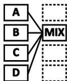
The four channels of an Axe-Fx II mixer are “wired” to the four grid rows in the column to the left of the mixer. In the first example at left, the level of Effect **A** would be controlled by the mixer’s CHANNEL 1 **LEVEL/GAIN** control, because **A** is on grid row 1. Effect **B** would be controlled by Channel 2, because B is on row 2, and so on.
