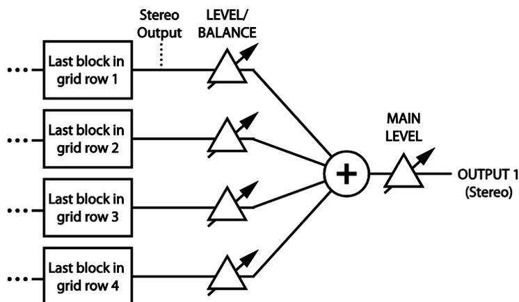
**LEVEL 1–4** – Think of these as input faders. Each is connected to one row of the grid as shown above.
