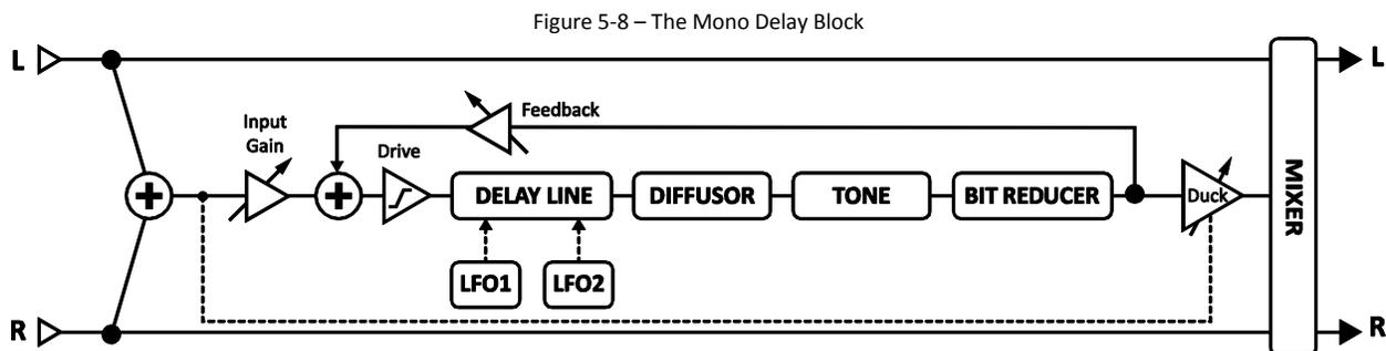
**TIME** – Sets the time of the delay in milliseconds. When **TIME** is shown in parenthesis, it is being set automatically by the **TEMPO** parameter (see below). Set **TEMPO** to “NONE” to regain manual control.
