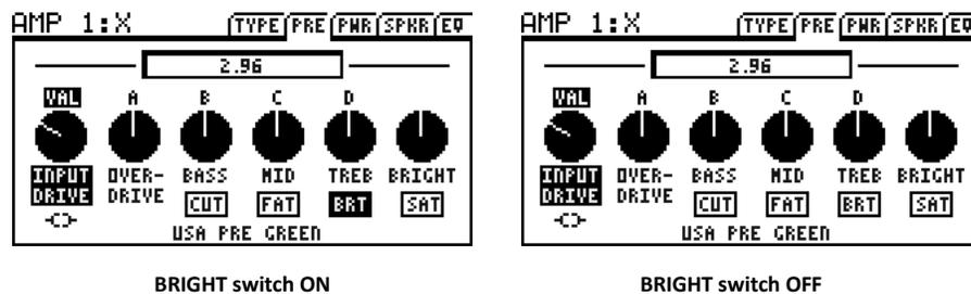
**CUT SWITCH** – (engaged by a switch beneath **BASS**) reduces the amount of low frequencies into the amp simulation. This can be used to achieve a “tighter” tone or to reduce low-end “flub”.
