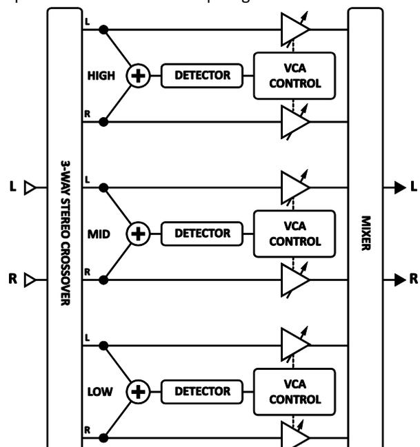
Figure 5-17 – Stylized view of the Multiband Compressor
