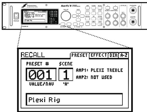
The **AXE-FX II** has 384 editable presets. Press **RECALL** to enter normal play mode. The **VALUE** wheel or **NAV** buttons select presets.
