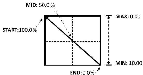
At first glance this seems to be a reversal of the example above, where pushing the pedal forward decreases the volume. But look closer and you'll find that **MIN** is set to "10.0" and **MAX** to "0.0". With both sets of values inverted, this setup sounds and works *exactly* like the one above!
