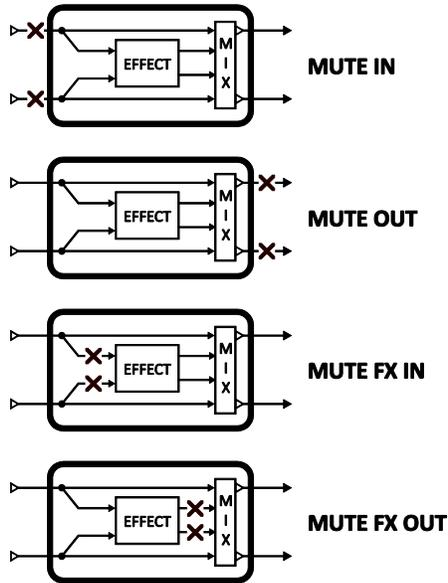
**MUTE IN** –When the block is bypassed, its inputs are disconnected, silencing the dry immediately but allowing existing effect “tails” to ring. New signals are prevented from entering the effect until it is re-engaged.
