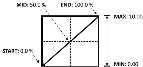
The default settings for **START**, **MID**, and **END** create a perfectly linear relationship between the source and the target. As the pedal is depressed, the volume increases in direct proportion. **MIN** and **MAX** are set to their extreme limits, so volume goes from 0.00-10.00 (OFF to FULL). But linear response is generally unsatisfactory for volume control because of the non-linear characteristics of our hearing. Ears aren’t very good at math...
