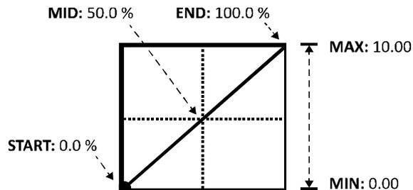
A now-familiar example: the default modifier setting for a **VOLUME** parameter, showing a linear sweep, with **MIN** and **MAX** set to their extremes.
