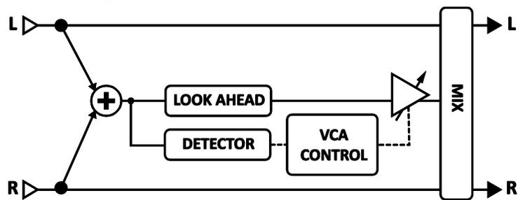
Figure 5-7 – The Compressor Block's "Studio" Type
