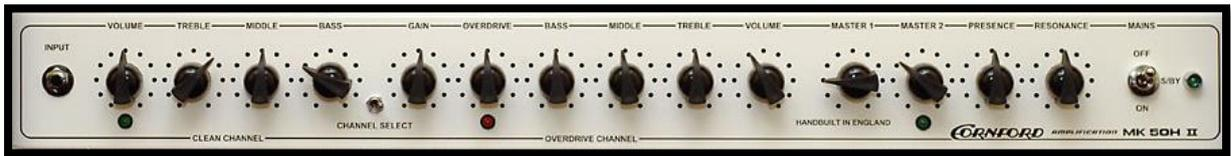
The amp has Master controls. This means that the amp's distortion is created in particular by the preamp tubes, not the power amp. The Master Volume, which works in the power amp section, is still very important to the tone and feel. You have to decide for yourself what setting in the amp model works for you best. The default setting is a good point to start.
