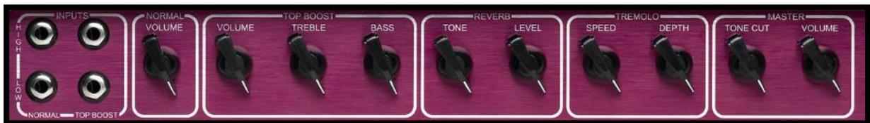
The AC30 has High and Low inputs per channel. If the original amp has High and Low inputs, the amp model is always based on the High input. To get the equivalent of the Low input, decrease Input Trim in the amp model.
