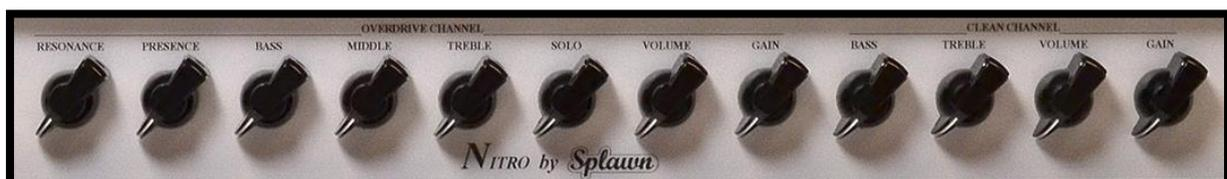
Controls on the amp: Resonance (amp model: Depth), Presence, Bass, Middle, Treble, Master, Gain.
