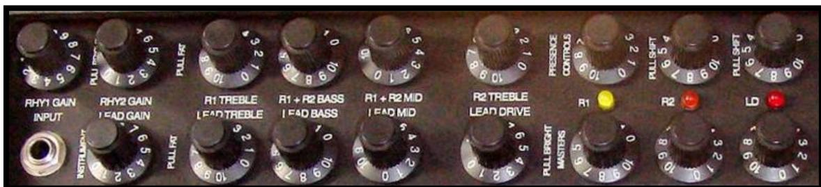
The amp's main controls are Gain, Bass, Mid, Treble, Presence and Master. "Pull" controls are:
