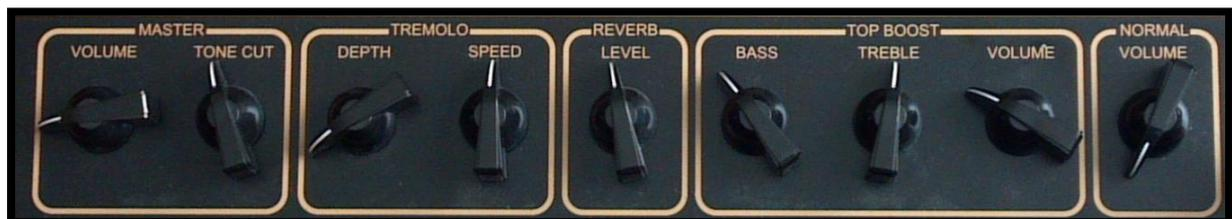
The original AC15 had two channels. The first channel provided a “Vibravox” effect (not modeled), a combination of tremolo and vibrato, plus Volume and Brilliance controls. Channel 2 had a Volume and a Cut control (amp model: Hi-Cut). Later models with Top Boost added Bass and Treble controls. **More recent models** offer Normal and Top Boost channels with additional options (Bright, Master Volume etc.).
