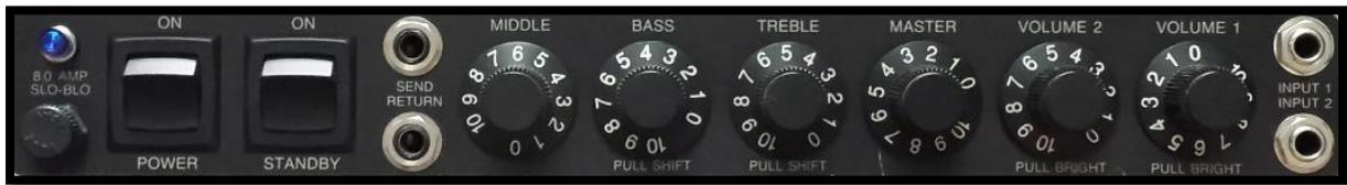
Controls on the original amp: Volume (pull: Bright, channel 1), Master, Bass (pull: Shift) , Middle, Treble (pull: Shift), 7-band GEQ.
