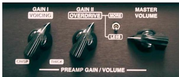
The MORE / LESS switch activates or defeats a tube gain stage. The interesting and often overlooked benefit of this switch is that you can use it in conjunction with the gain controls to tailor your tone as well as distortion amount. For example, set GAIN I, GAIN II, MORE/LESS and MASTER VOLUME as shown in the photo above and play for a few minutes. Now set these controls as shown in the photo below.
