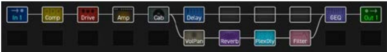
**Ex 4:** A complex preset with effects *before* and *after* two amps. A stereo cab feeds OUT 1 (Front of House), while Output 2 taps the signal with NO cab for use with a neutral power amp & real guitar speakers (on-stage backline).
