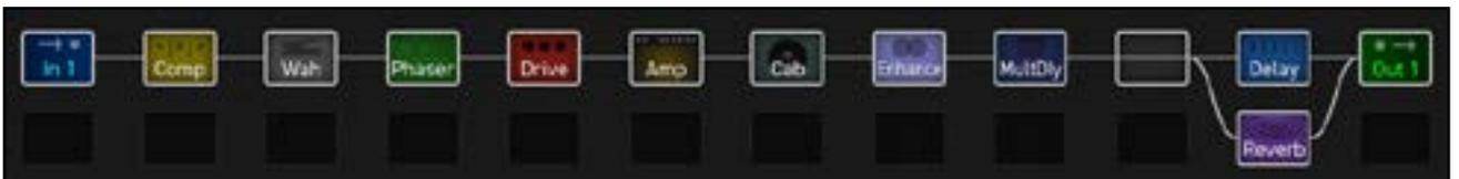
**Ex 3:** An entire parallel chain for a shimmering, filtered effect with a VOLUME block for its own "Send" control.
