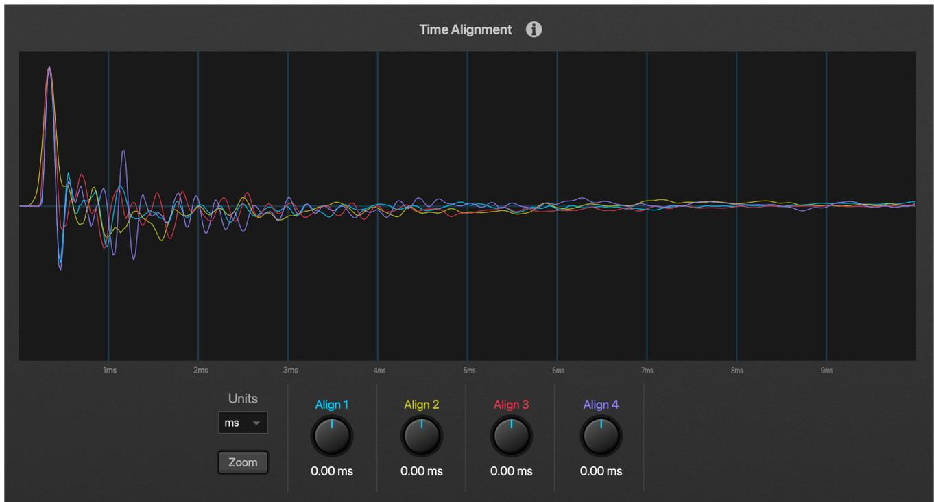
The Align view displays superimposed time domain plots for all the currently loaded IRs. Use the four correspondingly colored knobs to make adjustments, choosing either millimeters or milliseconds as desired
