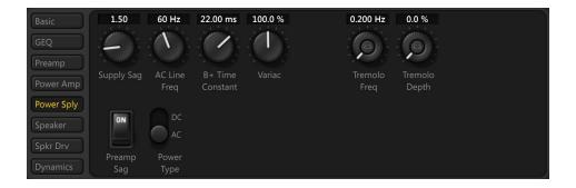
SUPPLY SAG – Controls power supply impedance. Higher settings simulate higher power supply impedance, causing greater tube plate voltage (B+) "droop" and giving a more compressed, spongy and looser feel. Sag interacts with the MASTER: as the power amp is pushed and draws more current from its power supply, Sag has more effect. Sag values around 2 simulate a solid-state rectifier, 4-6 a tube rectifier.
