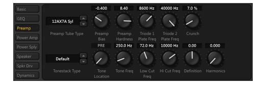
PREAMP TUBE TYPE – 12AX7A SYL is the default. The EF86 has been normalized to have roughly the same gain as the triode types.
