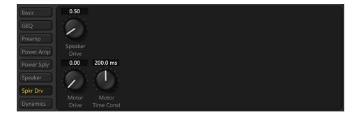
SPEAKER DRIVE – Simulates distortion caused by pushing a speaker too far. It interacts with the MASTER.
