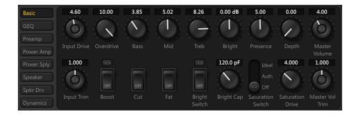
INPUT DRIVE – Also known as Drive, Volume, Gain, etc. It is the knob closest to the input jack. In many cases it has a bright cap so the frequency response will be dependent on the knob position. As the gain increases the tone shifts from a treble and upper mid emphasis to a bass and lower mid emphasis. On jumpered amps, this setting's label changes to TREBLE DRIVE.
