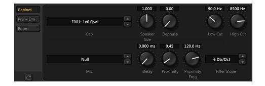
CAB – Loads a cabinet impulse response (IR). The older FAS and RW cabs were recorded with neutral mics. OH, Kalthallen, and the Mix/Producer Pack series have matching mics included in the IR.
