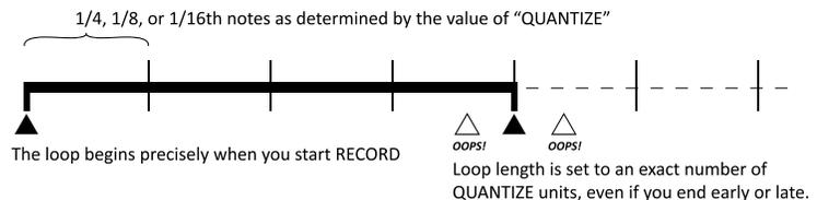
**RECORD BEATS** allows you to pre-determine the number of units. Recording ends and playback automatically begins when you reach the designated length (unless **PLAY IMMEDIATELY** is set to “OFF”; See below.)
