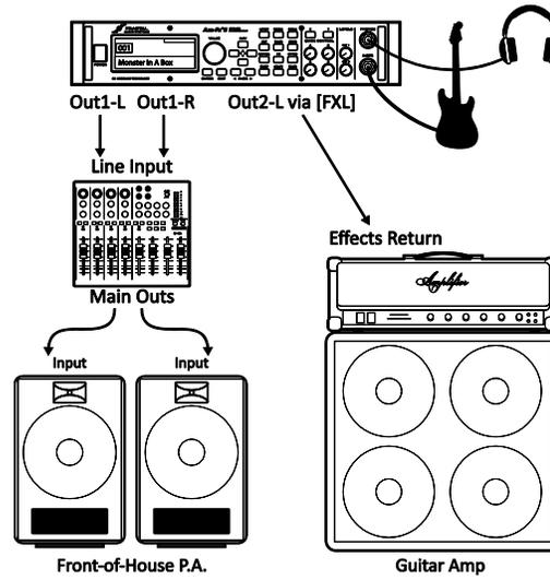
**Global Settings:** Default **I/O Settings:** Set OUT1 MODE and OUT 2 MODE as required for stereo or mono
