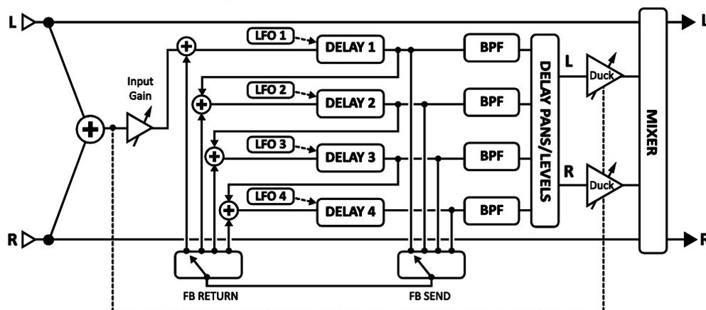
The parameters of the Quad Series Delay are identical to those of the Quad Tap delay (5.20.1 above), except for the absence of the diffusor block controls, the **FEEDBACK SEND** and **RETURN** parameters, and the single **FEEDBACK** control.
