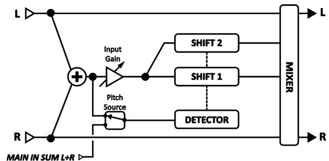
Figure 5-31 - The Octave Divider Pitch Shifter Type
