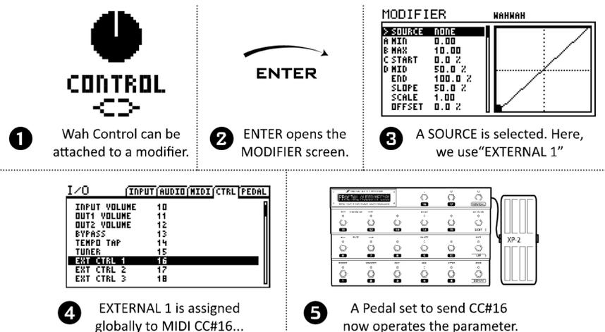
Let’s assume that the controller called “EXT 1” has already been set up (in the CTRL page of the I/O menu) for MIDI CC# 16 (its default setting), and that we have connected a MIDI foot controller with an expression pedal that is set up to send this same message on the correct MIDI channel. (In fact, this is the default setting for the EXPRESSION PEDAL 2 jack on the MFC-101).
