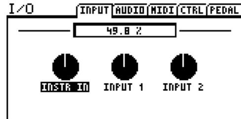
**!** Changing input levels will NOT affect *what you hear*. Inputs are *compensated*, meaning that as you lower trims to optimize signal-to-noise ratio going into the converters, the output of the converters is adjusted inversely so “what you hear” (and what reaches the signal processor) always *remains the same*.
