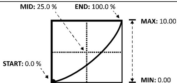
As we lower the value of **MID**, the response starts to take on a more comfortable curve, closer to the classic log or audio taper typically used for volume control. **MIN** and **MAX** are still set to “0.0” and “10.0” so that volume goes from off to full, but the way it *swells* has changed.
