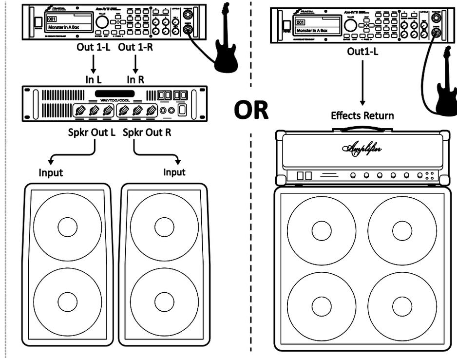
**Global Settings:** Power Amp Simulation **ON** or **OFF** (see below), Speaker Cabinet Simulation **OFF**
