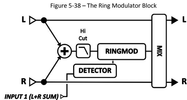
Each Axe-Fx II preset can use two fully independent **Ring Modulator** blocks.
