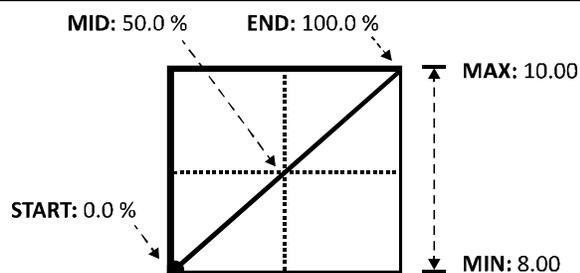
Unlike the preceding examples, this one does not show **MIN** and **MAX** set to their extremes. Instead, the range goes from 8.0 to 10.0, so our volume pedal will create only a small swell as it is rocked from heel to toe. You might use this to create a variable solo boost pedal.
