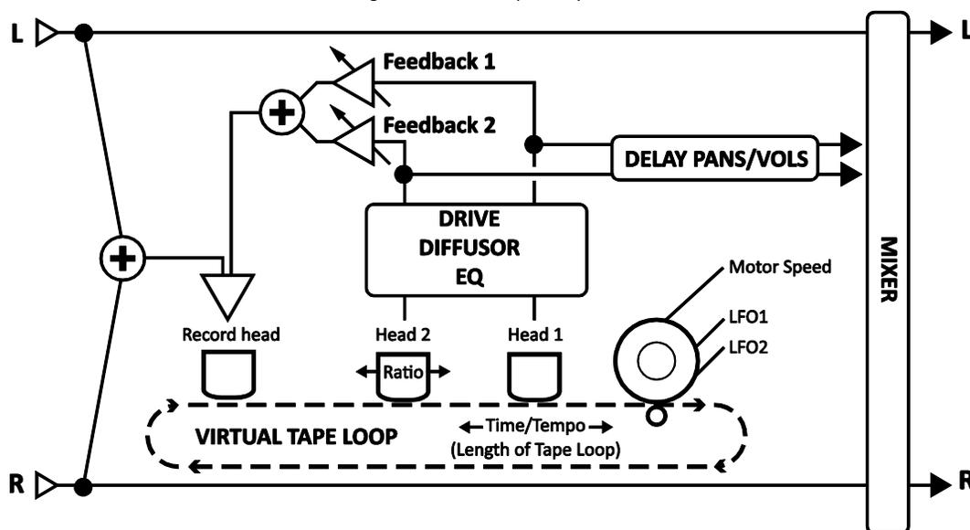
**MOTOR SPEED** – Sets the relative speed of the tape motor from 50% to 200%. This parameter can be modified in real time, making it possible to “timewarp” delayed material.
