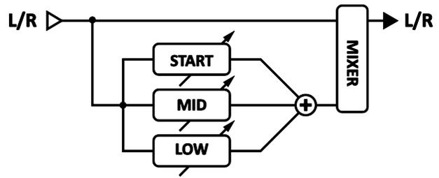
A formant filter is an extension of the wah principle but operates with a far more *vocal* quality. Formants represent particular resonances of instruments, or in this case, of the human vocal tract. The human vocal tract generates a handful of formants to produce the vowel sounds we recognize. For example, the vowel sound "eee" can be reproduced with a bank of narrow bandpass filters with various frequencies and amplitudes.
