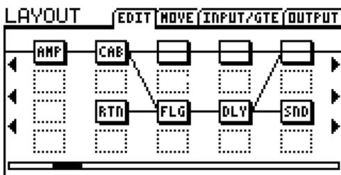
At left, the significant columns of this preset are shown as they would appear on the display of the Axe-Fx II. Notice that on the Axe-Fx II the connector from SEND to RETURN is *not visible*!
