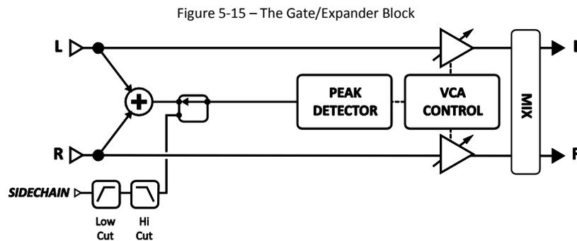
**THRSH** – (Threshold) Sets the level below which automatic volume reduction will occur. When input level is lower than the threshold, the expander reduces output volume as set by the **RATIO**.
