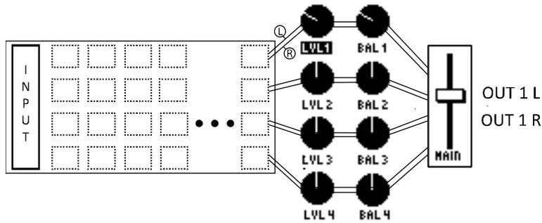
To review: channels 1-4 of the OUTPUT mixer are fed respectively by the stereo outputs of rows 1-4 of the grid. Each “channel” has a LEVEL that determines the gain of the incoming signal (+/- 20dB) and a BALANCE control that determines how the LEFT and RIGHT channels contribute to the final mix. A master GAIN slider offers +/-20 dB control over the final mixed output.
