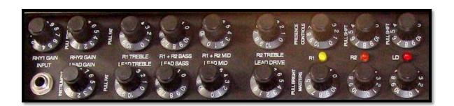
The amp's main controls are Gain, Bass, Mid, Treble, Presence and Master. "Pull" controls are:
