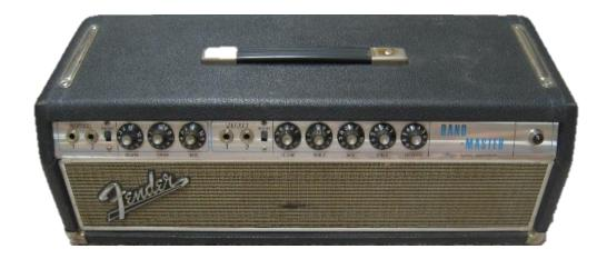
**Synopsis** Model of a '68 silverface Fender Bandmaster with blackface AB763 circuit,
