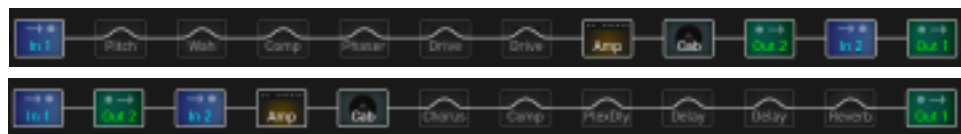
FM3 signal path showing the OUT 2 and IN 2 blocks positioned for POST FX (top) and PRE FX (bottom). You could also place additional FM3 blocks before or after the insert.
